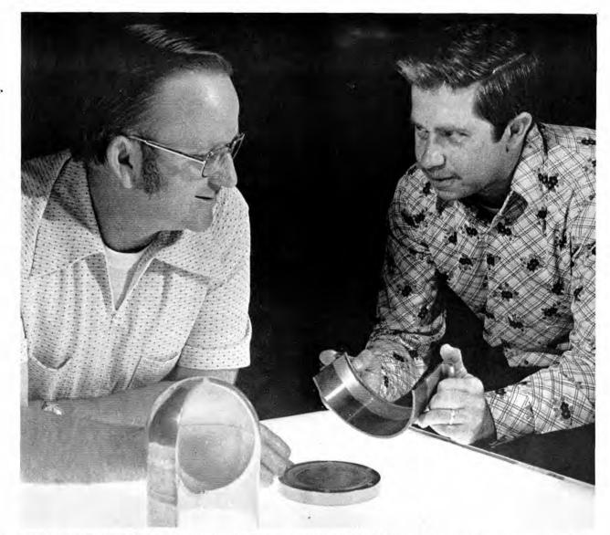
COMPULSIVE JOINERS— Rudy Johnson, left, and Jack Dini (both 8312) examine an electrochemically joined specimen of stainless steel and uranium . The two metallurgists have developed process for joining of materials previously not joinable.
